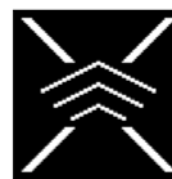
Fig. 04: Button symbol for acknowledging the warning tone
